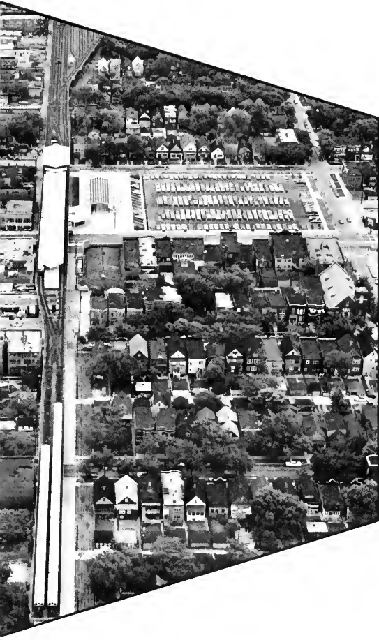
AERIAL VIEW looking east shows Englewood Extension facilities: (from foreground to background) tail track extending to Hermitage, Ashland station platform, transportation office building, bus terminal, parking lot, and expanded car storage yard.
